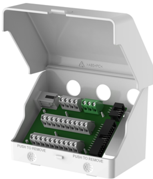
Fig. 1 Connection of the RS485 to USB on the connection box. GND connection not necessary
